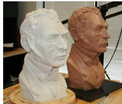
Original clay model and 3D Printed copy from 3D scan data
