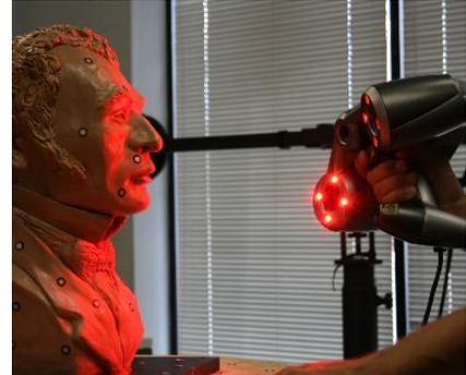
3D Scanning the clay model with a Creaform EXAScan 3D Scanner
