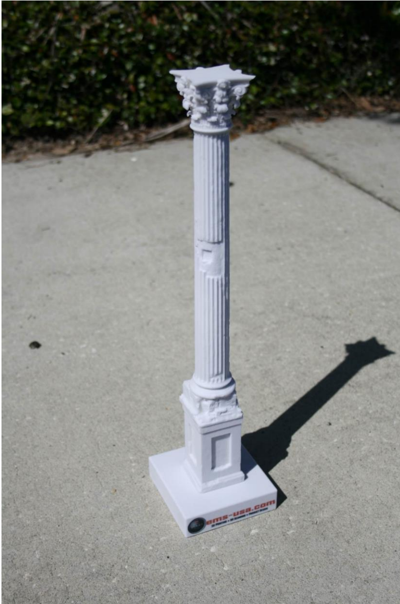
3D Printed scaled model from 3D Scan data
