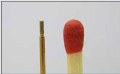
Point welded brass pin
