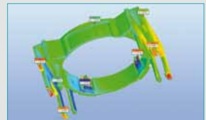
The nominal to actual comparison shows deviations between the manufactured part and the CAD model.
