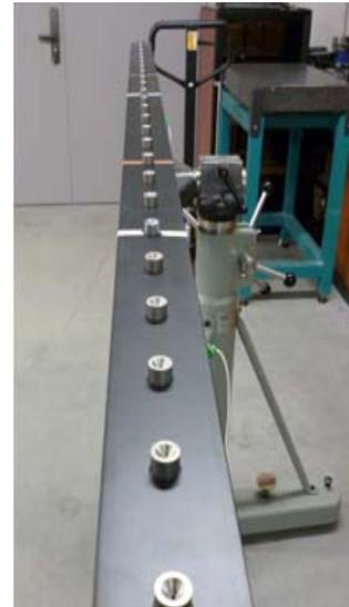
Figure 4: Verification artifact for VDI 2634 standard on its tripod [8]
