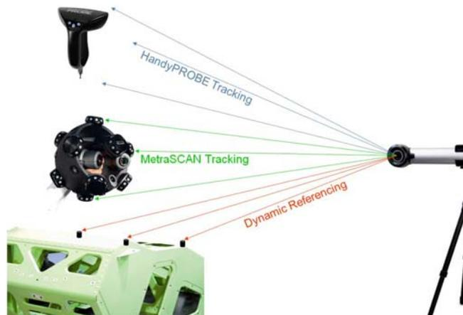
Figure 3: Operating principle of dynamic referencing
