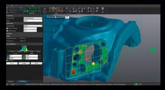
Use your 3D scan as a reference for your design: extract all the information you need from the mesh by creating geometrical entities, curves, cross-sections and even NURBS surfaces for characterizing freeform surfaces. The highly flexible, user-friendly VXmodel interface lets you quickly segment the mesh into all of the primitive entities required to complete the design in your CAD software.
