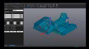
Before starting to reverse engineer the object, the scan must first be aligned to the coordinate system suiting your design requirements.
