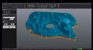
VXmodel will help you modify the 3D scan mesh, make it watertight and quickly generate print-ready files for your rapid manufacturing workflow.
